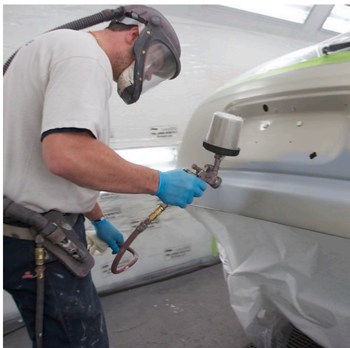
The MPCA has helped auto bodies shops in Minnesota reduce air pollution by adopting water-borne finish systems that work faster with less waste and energy consumption.
